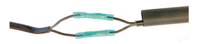
Step 10: Slide the Φ10mm heat shrinking tubing over the crimp terminals, tighten it by hot air gun
