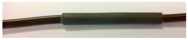
Please acknowledge that the fixed glue inside the shrinking tube, is coming out when heating, in order to close each tube end for the connection to be 100% water tight.
